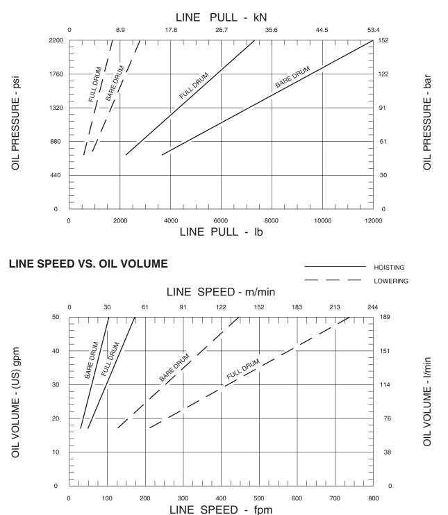
Performance graphs are based on standard hydraulic motor, gear ratio and cable drum with 5/8 inch diameter wire rope.
