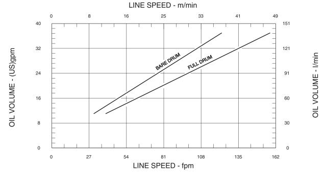
Performance graphs are based on standard hydraulic motor, gear ratio and cable drum with 1/2 inch diameter wire rope.
